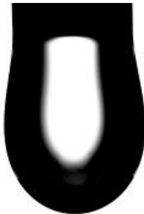
Fig. 6: Pendant drop of a contact adhesive at 120^\circ\text{C} .
