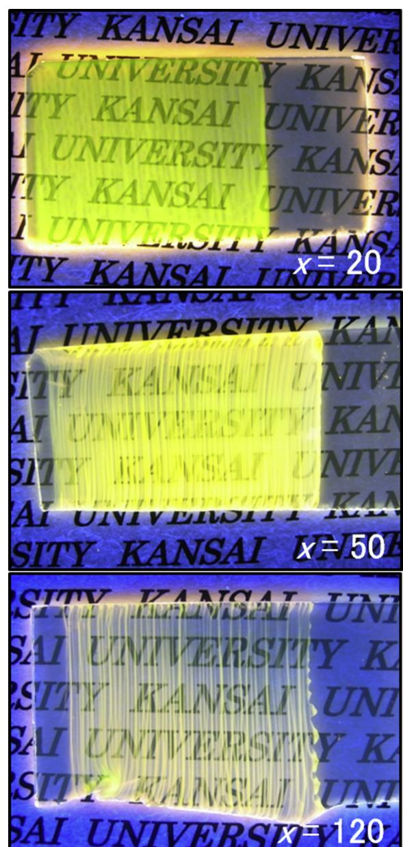
**Fig. 7.** Light emission from the R6G-doped silica-PVP hybrid films prepared at  $x = 20, 50$  and  $120$  under UV irradiation.
