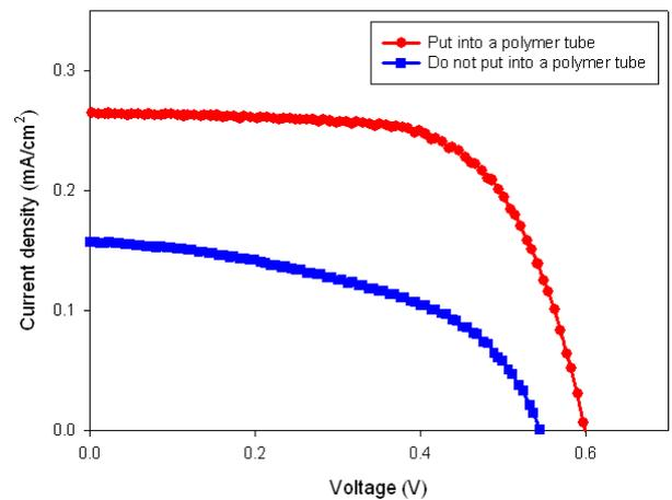
Fig. 6 I-V curves of the DSSCs fabricated with Zylon<sup>®</sup>
