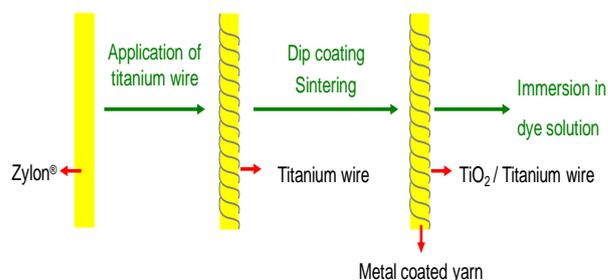
Fig. 2 A schematic of the cell applied Zylon® as an electrode
