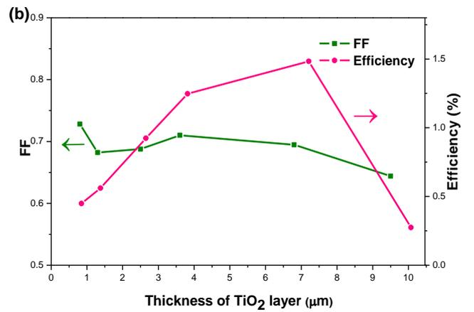
Fig. 5 Photovoltaic characteristics of fibrous DSSCs fabricated with various thickness of TiO<sub>2</sub> film; (a) V<sub>oc</sub> and J<sub>sc</sub> and (b) FF and Efficiency
