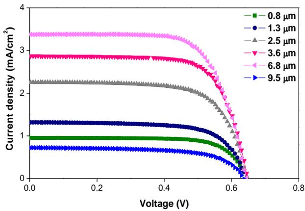
Fig. 4 I-V curves of fibrous DSSCs fabricated with various thickness of TiO<sub>2</sub> film
