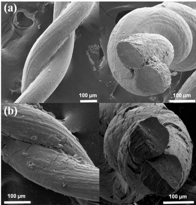
Fig. 3 SEM images of Ti wire coated with various TiO<sub>2</sub> film thicknesses; (a) TiO<sub>2</sub> layer thickness - 0.8 μm and (b) TiO<sub>2</sub> layer thickness - 9.5 μm.
