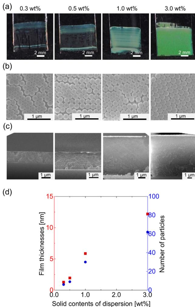
**Fig. 4.** (a) Photographs, (b) SEM images, and (c) cross-section SEM images of structural color films from  $\text{PSt}_{240}@\text{PDA}_4$  core-shell particles (lifting speed:  $0.1 \mu\text{m}/\text{s}$ ) with different solid contents. (d) Average film thickness and number of particles.
