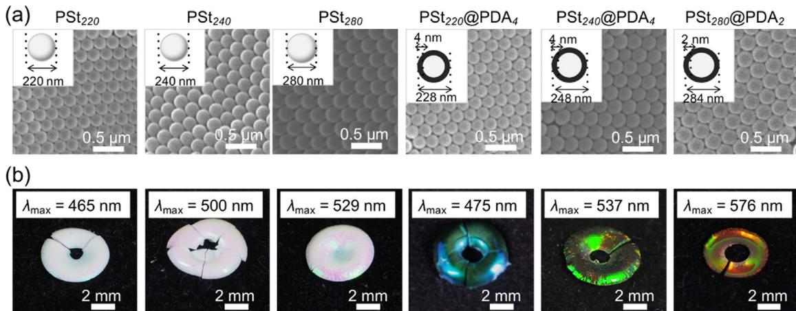
**Fig. 1.** (a) SEM images of core PSt particles (PSt<sub>220</sub>, PSt<sub>240</sub>, and PSt<sub>280</sub>) and core-shell particles (PSt<sub>220</sub>@PDA<sub>4</sub>, PSt<sub>240</sub>@PDA<sub>4</sub>, and PSt<sub>280</sub>@PDA<sub>2</sub>). (b) Structural color pellets from core PSt and core-shell particles shown in Fig. 1a. Insets show the  $\lambda_{\max}$  of reflection peaks.
