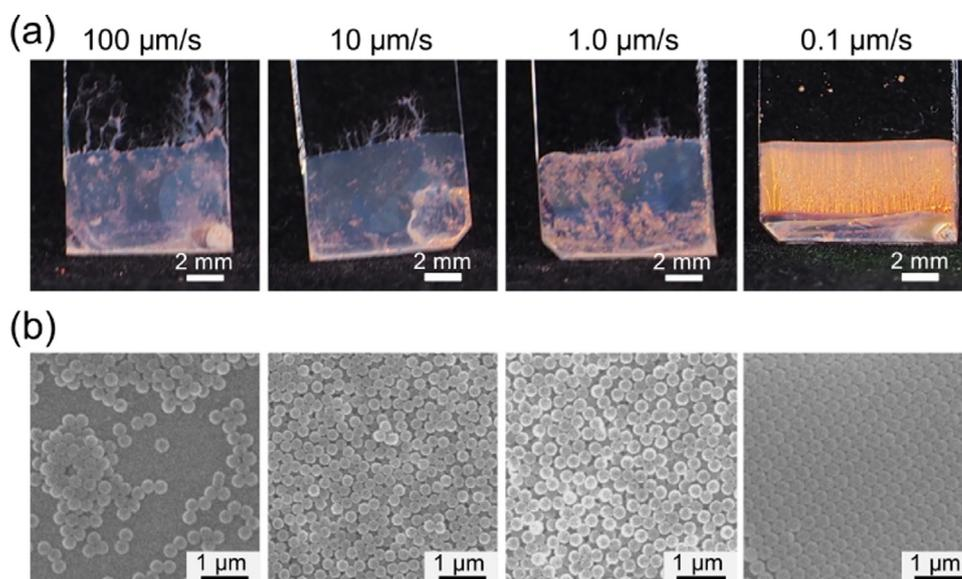
**Fig. 2.** (a) Photographs and (b) SEM images of structural color films from PSt<sub>280</sub>@PDA<sub>2</sub> core-shell particles (solid content of dispersion: 3.0 wt%) with different lifting speeds.
