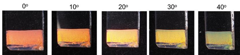
**Fig. 3.** Digital camera images of structural color films from PSt<sub>280</sub>@PDA<sub>2</sub> core-shell particles (solid content of dispersion: 3.0 wt%) at various angles.
