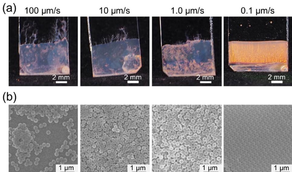
**Fig. 2.** (a) Photographs and (b) SEM images of structural color films from PSt<sub>280</sub>@PDA<sub>2</sub> core-shell particles (solid content of dispersion: 3.0 wt%) with different lifting speeds.
