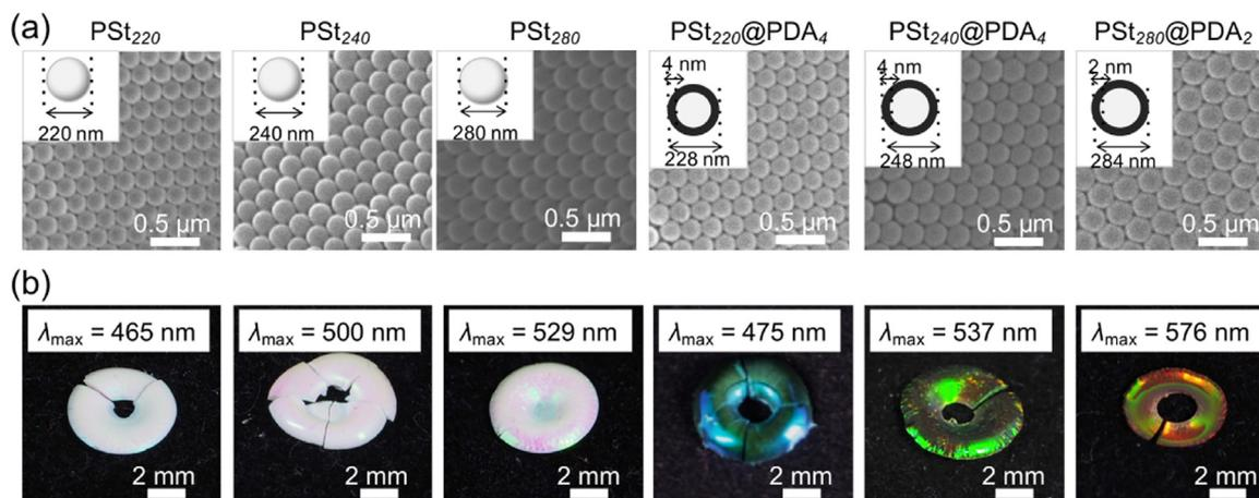
**Fig. 1.** (a) SEM images of core PSt particles (PSt<sub>220</sub>, PSt<sub>240</sub>, and PSt<sub>280</sub>) and core-shell particles (PSt<sub>220</sub>@PDA<sub>4</sub>, PSt<sub>240</sub>@PDA<sub>4</sub>, and PSt<sub>280</sub>@PDA<sub>2</sub>). (b) Structural color pellets from core PSt and core-shell particles shown in Fig. 1a. Insets show the λ<sub>max</sub> of reflection peaks.
