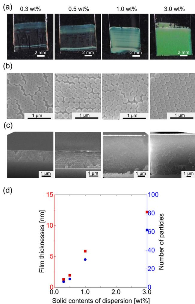
**Fig. 4.** (a) Photographs, (b) SEM images, and (c) cross-section SEM images of structural color films from PST<sub>240</sub>@PDA<sub>4</sub> core-shell particles (lifting speed: 0.1 μm/s) with different solid contents. (d) Average film thickness and number of particles.
