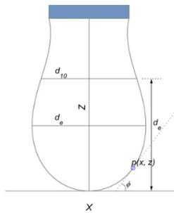
$$\Delta p = \gamma \left( \frac{1}{R_1} + \frac{1}{R_2} \right)$$
